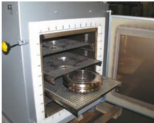
Air circulation furnace with charging grill shelves. The shelves can be moved individually on telescoping guides and can be taken out individually.
