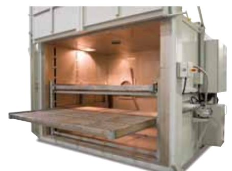
Drawer system for charging the furnace on several levels.
