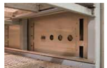
The openings for the vacuum and measurement connections of an air circulation chamber furnace
